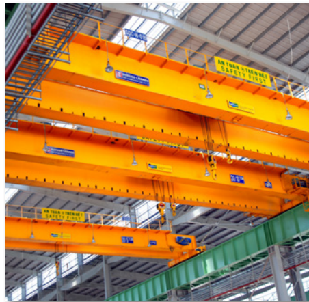
Double Overhead Hoist Crane
